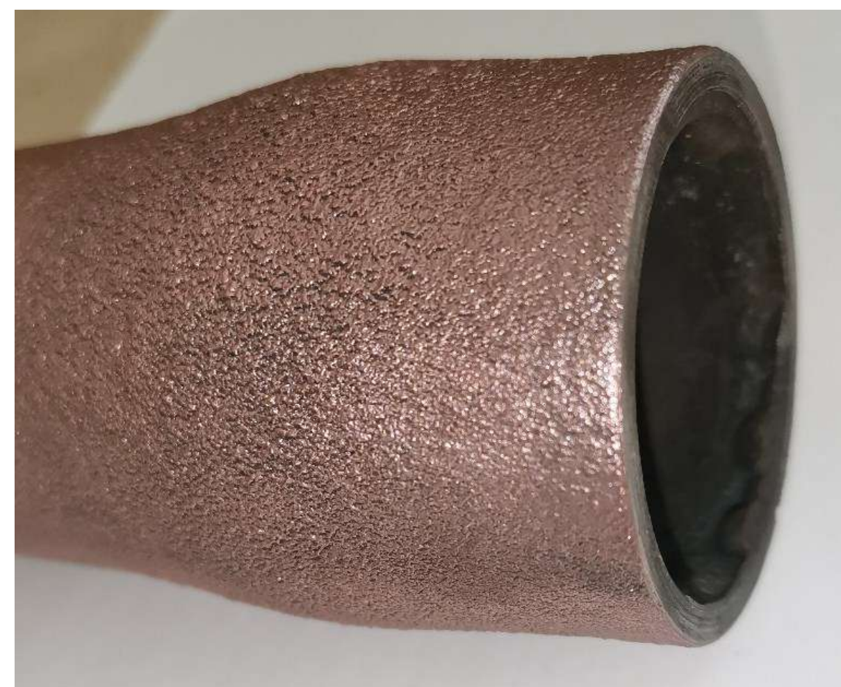
Fig.1. An example of a bronze product formed by plasma metallization
