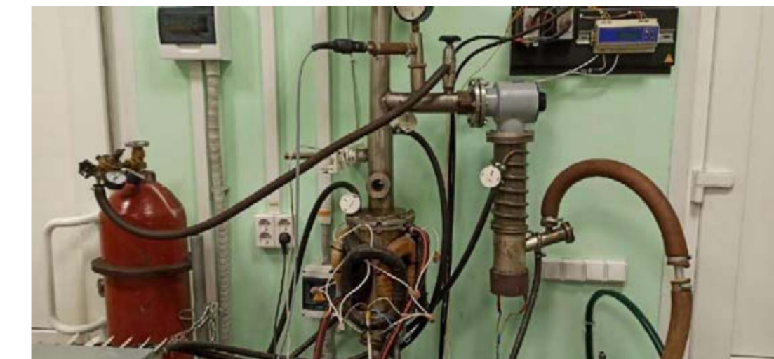
Experimental installation for electrical resistivity measurements
