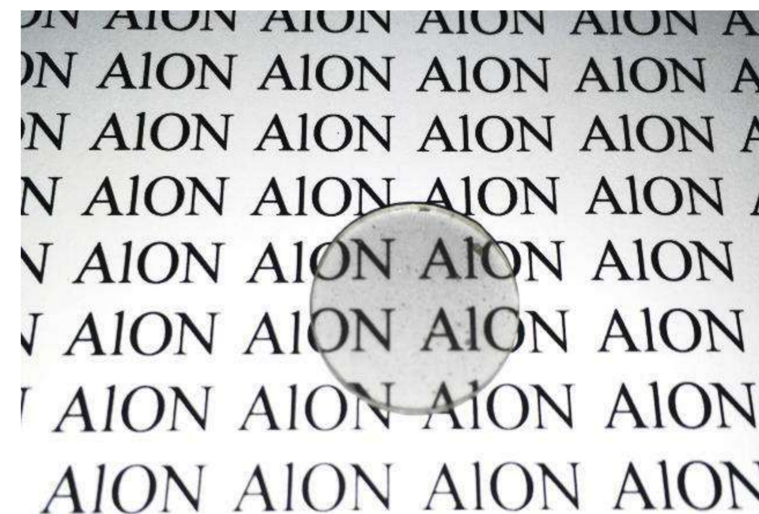
Figure 5. The image of AION transparent samples (a) and their light transmittance (b).
