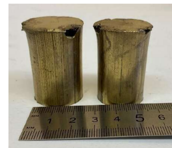
Fig. 2. The appearance of the preserved bronze samples after impact with the flyer-plate
