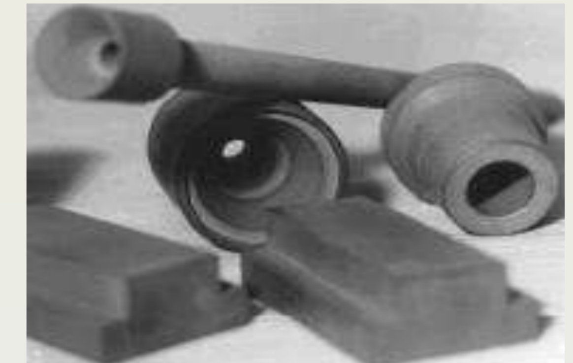
Fig. 2. Items made of CSed HMCCs: crucibles, nozzles for metal pouring and lining plates.
