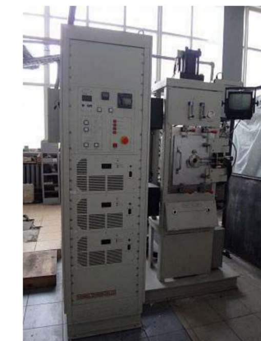
Figure - 12. Equipment SPS 10-3 for diffusion welding in vacuum (10 -4 Torr).
