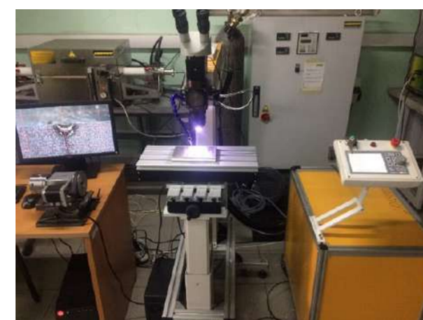
Figure - 4. Equipment for laser welding of the LAT-S-300 series.
