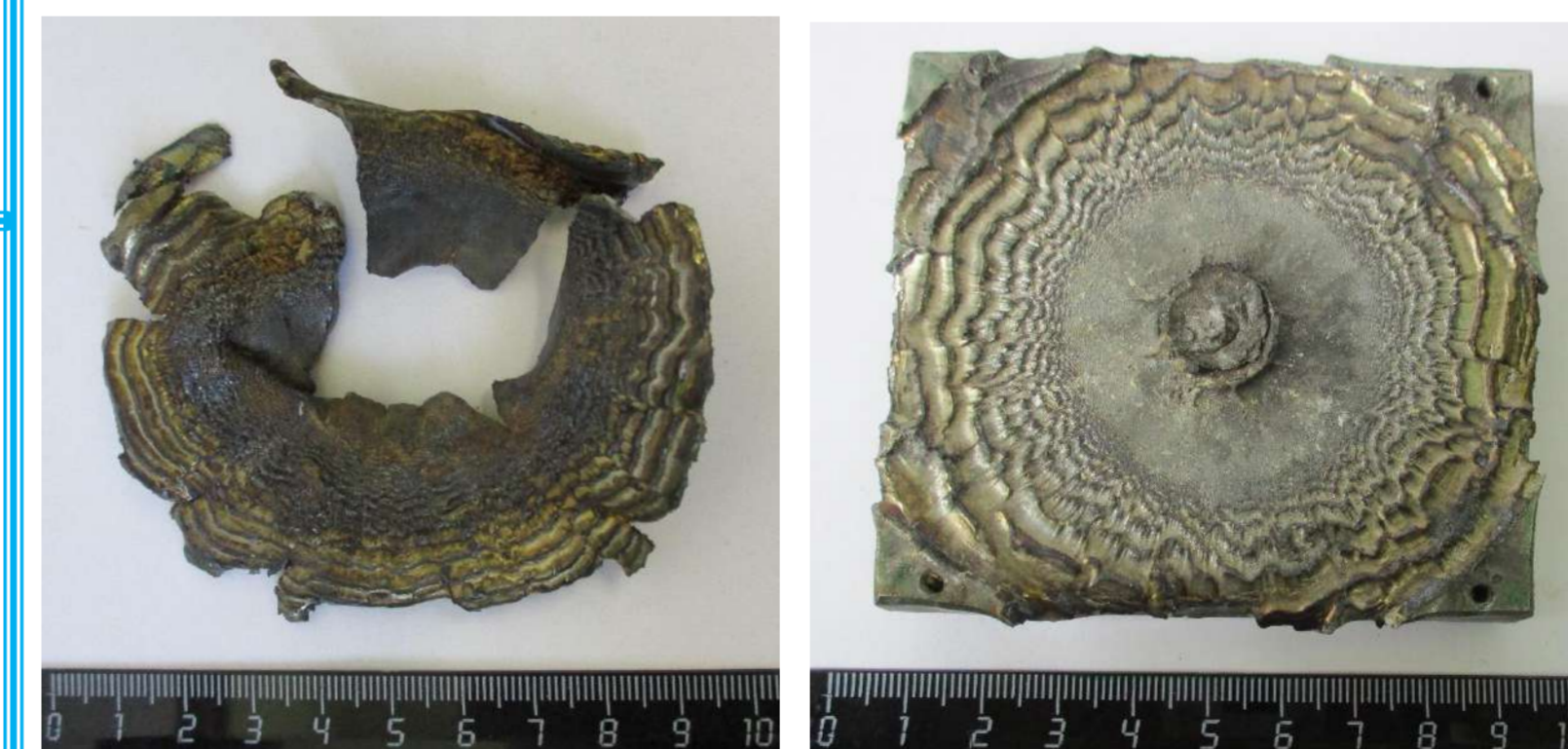
The bottom steel plate after shock-wave loading according to the first scheme
