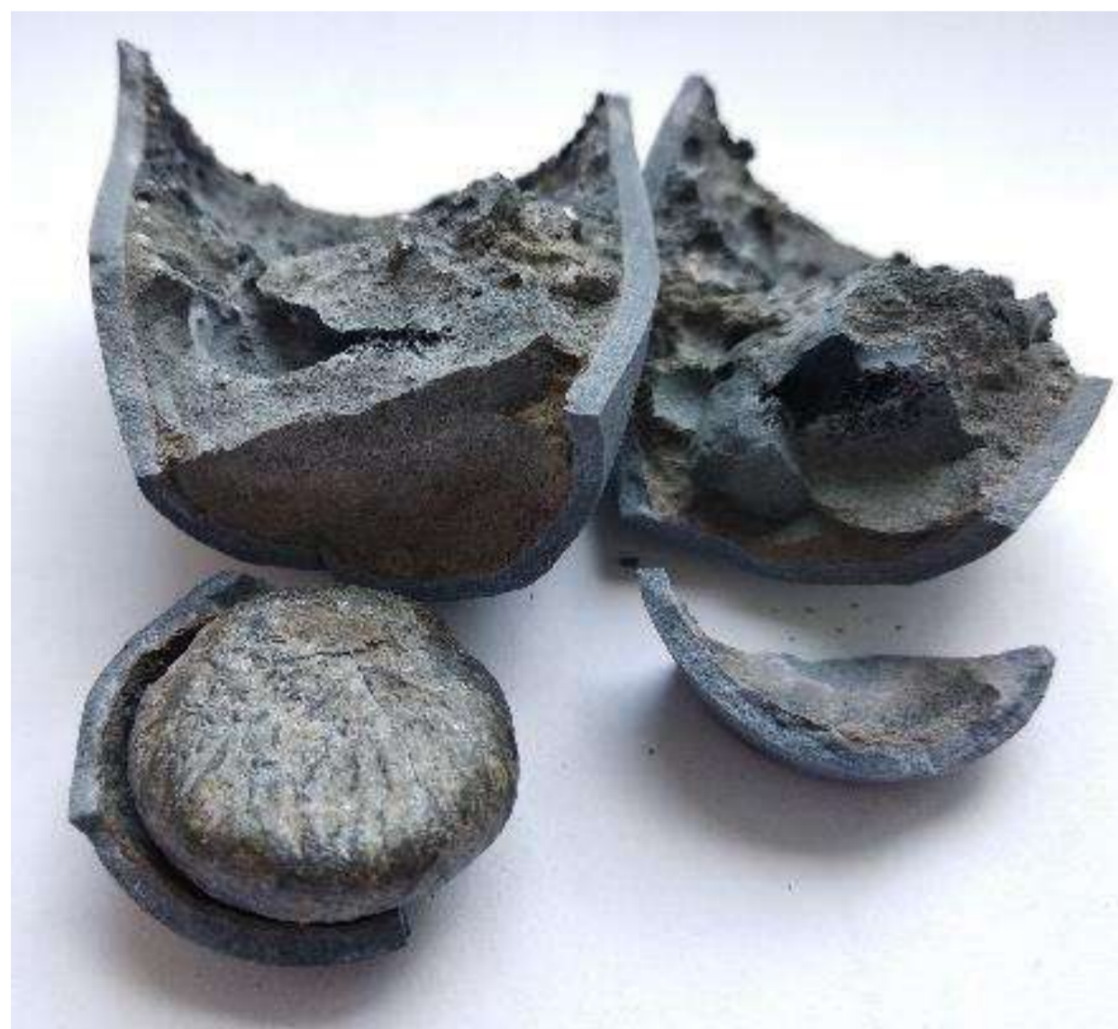
Fig.1 Results of melting oxides in an alund crucible
