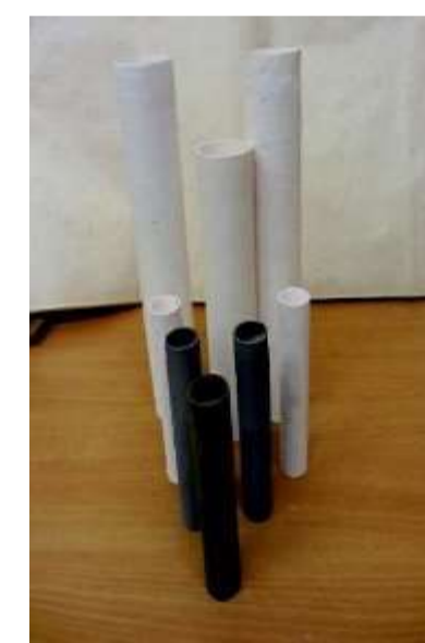
15. Porous capillary-permeable diaphragms (CPD) for electrochemical reactors (ECR) without and with functional thin-film (ion-plasma, magnetron) coatings for Izumrud and AQUAEHA installations
