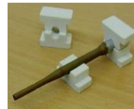
11. Electrical insulators for automatic bimetal welding
