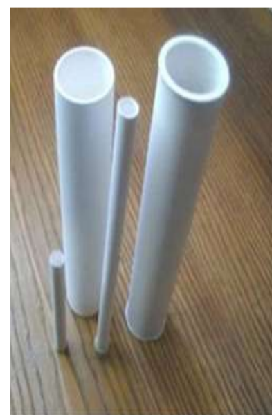
15. Porous capillary-permeable diaphragms (CPD) for electrochemical reactors (ECR) without and with functional thin-film (ion-plasma, magnetron) coatings for Izumrud and AQUAEHA installations
